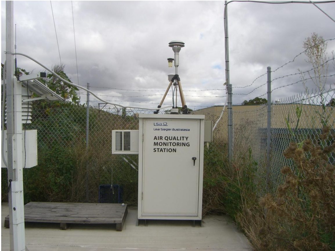
Figure 4 Southern weather & air quality monitoring station at ILC Site
