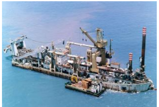
Figure 4: Cutter Suction Dredge Leonardo Da Vinci
