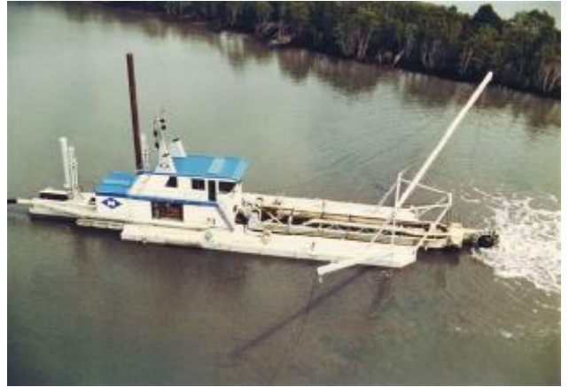
Figure 3: Cutter Suction Dredge Nu Bounty and departed in February 2009 (Figure 3). The 'Leonardo Da Vinci' (Figure 4) arrived in February 2009 departed in April 2009. The 'De Bougainville' (Figure 5) will arrive in June 2009 and will leave in approximately August 2009. The 'Marco Polo' (Figure 6) will arrive in approximately August 2009 and will remain until the completion of dredging, being approximately March 2010.
